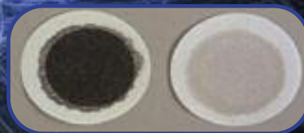
A fuel stability test showed typical heating oil (left) and heating oil after treatment with Oakley's VBA (right)
